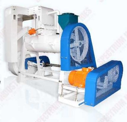
Capacities range from 250 kgs per hour to 4000 kgs per hour. When the parchment is fed at the right moisture content, the machines produces green coffee without beanbreakage and with uniform degree of polishing.
