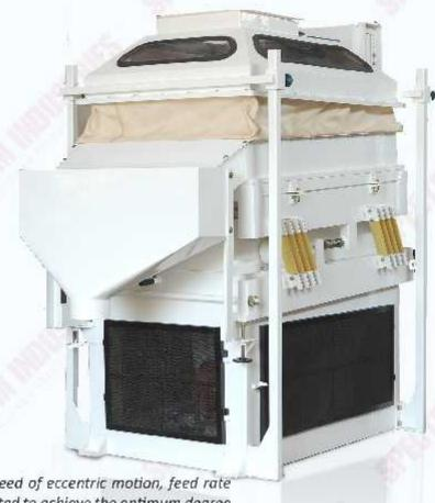
The inclination of the vibrating deck, speed of eccentric motion, feed rate and the air flow can be individually adjusted to achieve the optimum degree of separation. A wide variety of deck screens are available to suit specific applications.
