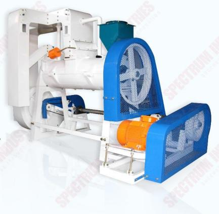
Capacities range from 250 kgs per hour to 4000 kgs per hour. When the parchment is fed at the right moisture content, the machines produces green coffee without beanbreakage and with uniform degree of polishing.
