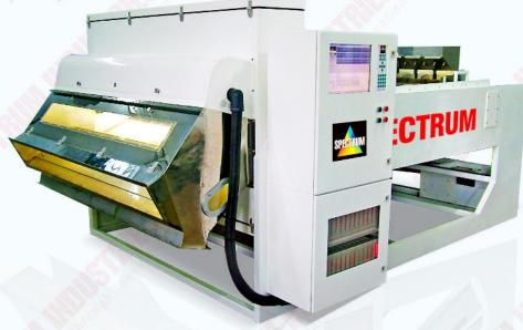
Large Format Lenses with digital automatic LED backlights are employed to ensure highest quality imaging of the product, that is also displayed on a 15" Colour LED TFT screen, for online viewing and monitoring of the product. The resultant data is compared with pre-set parameters, to reject the defective product using ultra-fast, long life, custom designed pneumatic ejectors.
