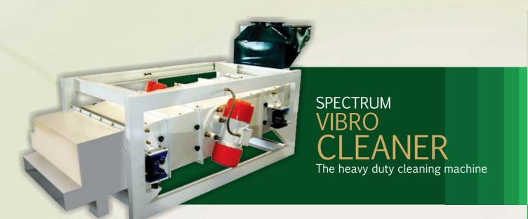
Spectrum Vibro-Cleaners are used for removing large impurities like stick, buck and leaves as well as fine dirt and sand from good product in seed cleaning and processing plants. They are provided with two vibrating screens, the top screen removes oversize material while the bottom screen eliminates fine dirt and sand.
