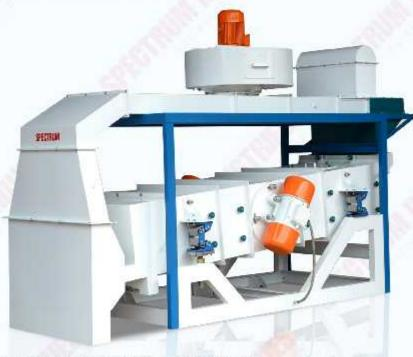
The deck inclination, stroke and angle of throw are adjustable for optimum performance. Automatic Screen cleaning is provided by means of the Rubber ball tray system that ensures consistent and effective cleaning of the screens. The Screens are easily removable and the machine is provided with a swing down type door for easy access and change or cleaning of screens.
