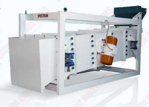
The screens can easily be changed by swinging down the inlet door and sliding them out
